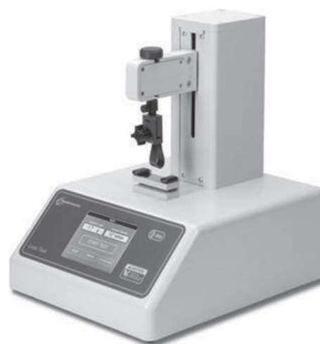
Fig. 7. Loop Tack 2000 (LT-2000) device is used to determine the loop tack of self-adhesive materials [4].
